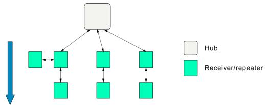
Power up and pair the radiator actuators and thermostats, from the furthest from the hub to the closest to the hub.
